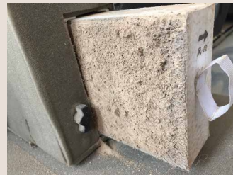
Dirty PM 2.5 Filter after 1 month field test
