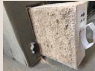
Dirty PM 2.5 Filter after 1 month field test
