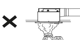
■ When the ceiling is unable to dismantle, please set a square inspection hole of at least 45 cm. (The inspection hole should not be directly under the duct pipe.)
