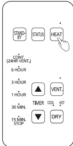
① Press the **HEAT** button to start the heating mode.
