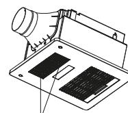
Left and right air outlet grilles can be adjusted in 4 directions.
