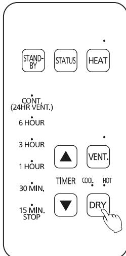
\* The indicators of COOL or HOT, and default setting time (15 MIN.) light on, then turn off automatically after 3 seconds.
