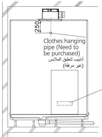
To make the effect of drying clothes better, you are recommended to set a ventilation shutter at the lower part of the door with a valid opening area of 100 cm<sup>2</sup> or above.
